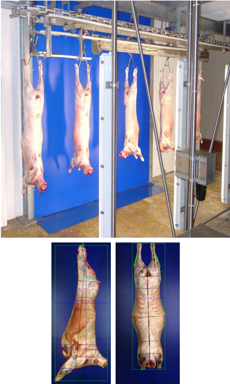
Fig. 8. Video image analysis of lamb carcasses with an E+V Technology VSS2000 system.
